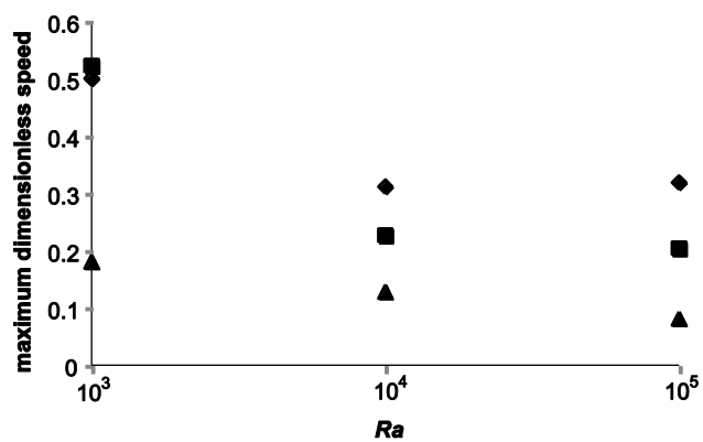
Figure 6. The maximum dimensionless speed at steady state for the nine stable cases, close to the explosion boundary, described in Table 2. The diamonds represent those cases with Bi = 100 , the squares are cases with Bi = 10 and the triangles are those with Bi = 1 .
