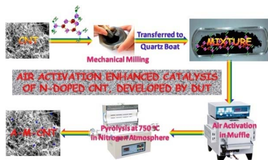
Scheme 1 Schematic illustration for the fabrication of novel nitrogen-doped carbon nanotube (A-M-CNT) through a facile PAA-PM approach.
