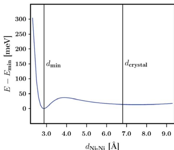
**Figure 6** Relative energies of two DUT-8(Ni)<sub>open</sub> M3 molecules for an increasing distance  $d_{\text{Ni-Ni}}$  between them. The free Ni sites are facing each other.  $E_{\text{min}}$  is the energy minimum for the imposed magnetic ordering.
