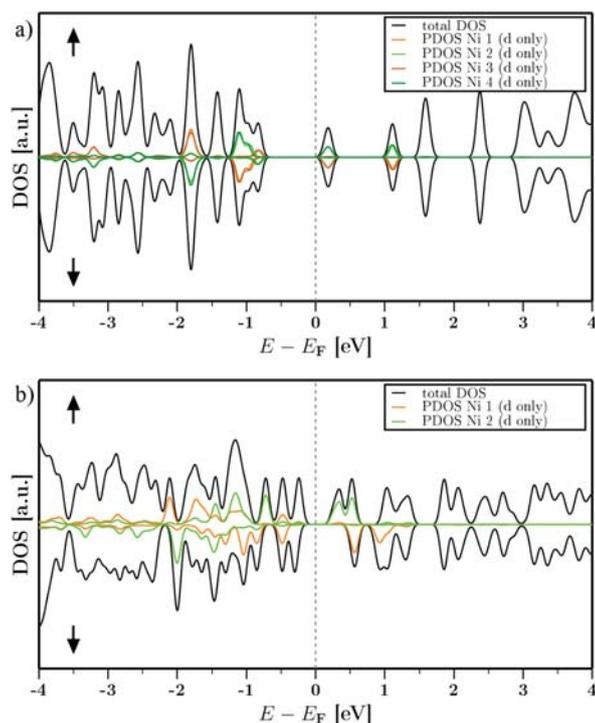
**Figure 5** Density of states, splitted into spin up ( $\uparrow$ ) and spin down ( $\downarrow$ ) densities, for a) DUT-8(Ni)<sub>open</sub> and b) DUT-8(Ni)<sub>closed</sub>. States with energies around the Fermi level  $E = E_F \pm 4$  eV are displayed.
