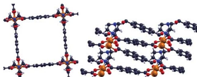
**Figure 1** Comparison of the tetragonal DUT-8(Ni)<sub>open</sub><sup>12</sup> (along  $\vec{c}$ ) and the triclinic DUT-8(Ni)<sub>closed</sub><sup>13</sup> (along  $\vec{b}$ ) (four Ni dimers are displayed in each structure for comparison).
