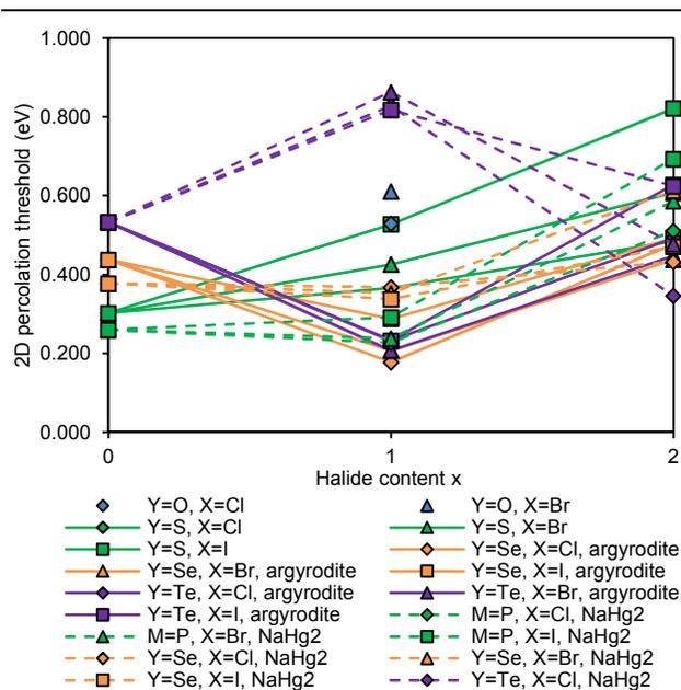
Fig. 17 Activation energies for  $\text{Li}^+$  migration in compounds containing different  $\text{Y}^{2-}$  anions.
