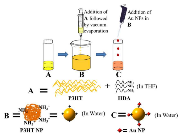
Scheme 2: Schematic representation of preparation of P3HT PNPs/ Au NPs composite
