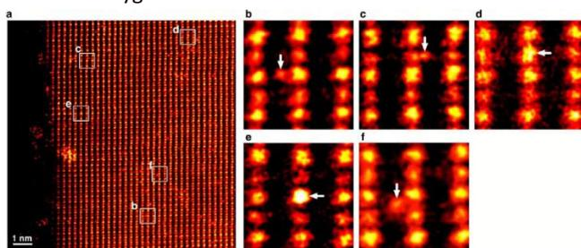
**Figure 5.** Atomic-resolution STEM images of platinum single atoms on a  $\text{TiO}_2$  (110) surface. (a) The overview. (b-f) The local enlargement of five Pt single atoms located at various surface sites on the unit structure. Copyright 2014 American Chemical Society.
