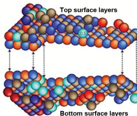
**Figure 7.** Overview of the two surface layers of a MgO crystal, as deduced from a dedicated aberration-corrected HRTEM image. The lattice sites, half-occupied sites, and Mg:O site ratio are clearly visualized. Copyright 2014 Nature Publishing Group.
