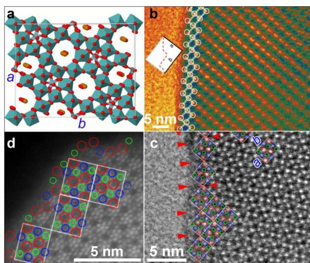
**Figure 1.** Surface structure of the complex M1  $\text{MoVTenbO}_x$  catalyst. (a) Crystallographic model of the M1 phase. (b,c) HRTEM images of one M1 nanoparticle along the  $\langle 001 \rangle$  direction far from (b) and near (c) the Scherzer focus. (d) STEM image. Copyright 2010 John Wiley and Sons.
