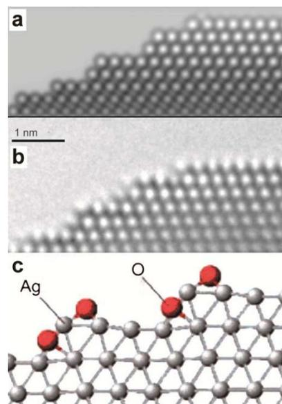
**Figure 3.** Surface elucidation of a Ag catalyst nanoparticle. (a) High-resolution simulated image. (b) HRTEM image. (c) Model representation. Copyright 2008 John Wiley and Sons.
