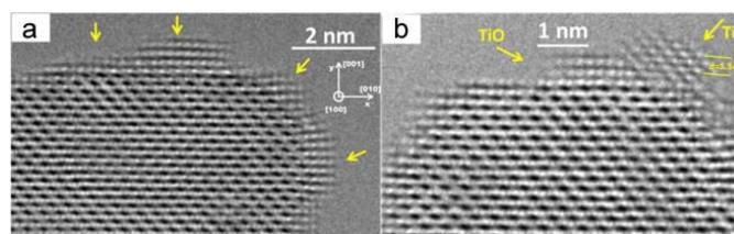
**Figure 2.** Real-space observation and comparison between TiO and Ti islands on a SrTiO<sub>3</sub> surface. (a) TEM image of TiO islands. (b) TEM image of a Ti island beside a TiO island. Copyright 2015 Elsevier.
