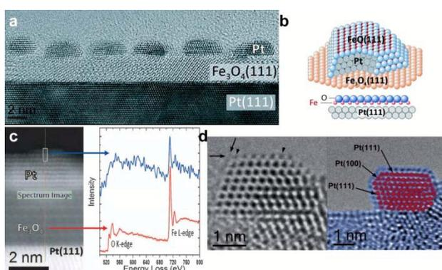
**Figure 8.** Pt/Fe<sub>3</sub>O<sub>4</sub>(111) model catalyst. (a) The overview HRTEM image. (b) Model representation of the SMSI FeO(111)
