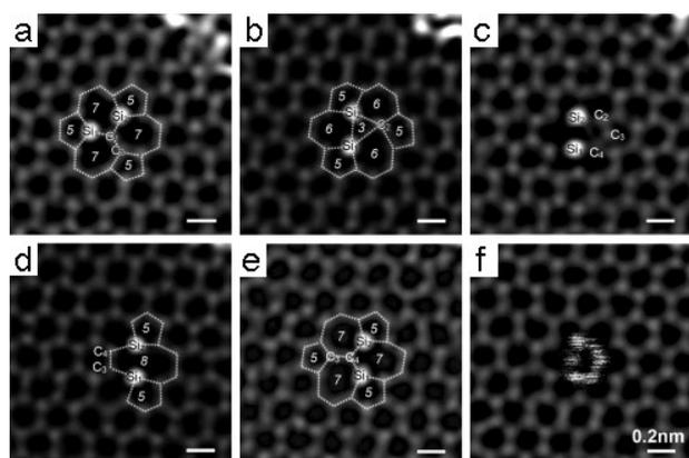
**Figure 6.** Formation of a silicon trimer at 80 kV was dynamically recorded in monolayer graphene with atomic resolution, showing the lattice dynamics process (a-f). Copyright 2014 John Wiley and Sons.
