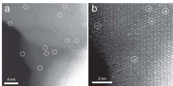
**Figure 4.** Atomic-resolution STEM images of platinum single-atom catalyst supported on an  $\text{FeO}_x$  surface. Pt single atoms, illustrated by white circles, are uniformly dispersed (a) on the support and (b) further exactly occupy the Fe-atom positions. Copyright 2011 Nature Publishing Group.
