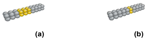
Fig. 5 Snapshot of the NW-4C nanowire of length l = 10 at c = \tilde{c}_\alpha (a) and c = \tilde{c}_\beta (b) in the canonical ensemble at T = 400 K. Cu atoms are in yellow and Ag atoms are in grey.
