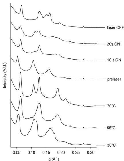
Figure 8 SAXS scattering data for POPE and PEG-lipid system in excess water with 3 nM GNR at equilibrium temperatures (30, 55 and 70°C) and after irradiation with the laser.
