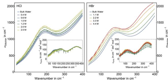
**Fig. 1** Concentration dependent THz/FIR absorption of aqueous  $\text{HCl}$  (left) and  $\text{HBr}$  (right) solutions. Each data point was obtained as the average of several measurements. The insets show the ionic extinction. In both panels a certain color represents identical concentrations.
