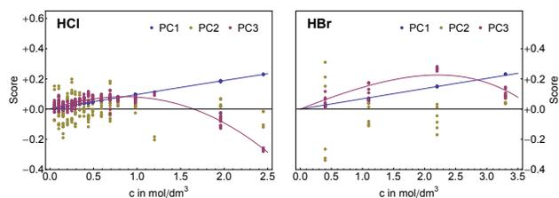
**Fig. 3** Concentration dependency of the scores of the first three principal components for aqueous HCl (left) and HBr (right) solutions. The first principal component (blue) shows mostly linear behavior, while the non-linearity of the third (red) principal components is indicative of ion pair formation. The second principal component (yellow) describes residual water vapor absorption in the beam path and is independent of the solute concentration.
