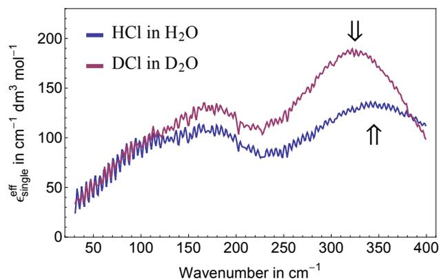
**Fig. 5** Comparison of the effective ionic extinctions of HCl in H<sub>2</sub>O and DCl in D<sub>2</sub>O showing a redshift of the high frequency resonance around 340 cm<sup>-1</sup> when replacing H by the heavier isotope.
