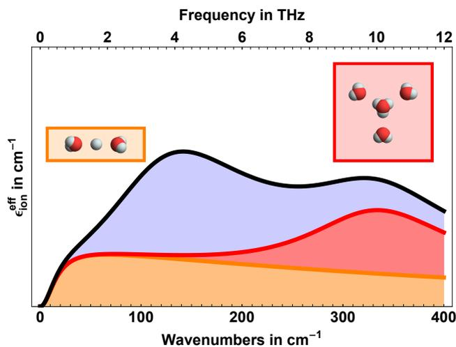
**Fig. 8** Zundel (orange), Eigen (red) and hydration water (light blue) contributions to the THz/FIR extinction of the solvated proton
