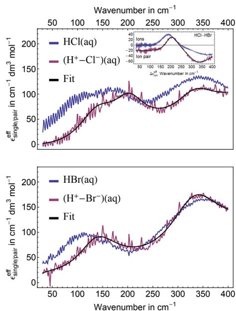
**Fig. 6** Comparison of single ion and ion pair extinction spectra for HCl (top) and HBr (bottom). The inset in the top panel shows the extinction differences HCl–HBr for single ions (in blue) and ion pairs (in red).
