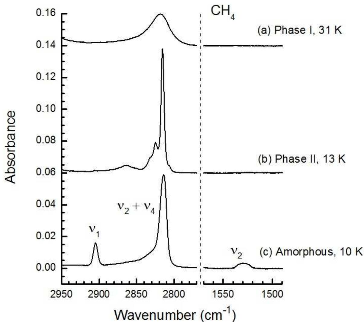
**Fig. 2** Infrared spectra around the  $\nu_1$  band near  $2904\text{ cm}^{-1}$  (left) and the  $\nu_2$  band near  $1530\text{ cm}^{-1}$  (right) for the three phases of solid CH<sub>4</sub> studied. Spectra are shown for samples with a thickness of  $\sim 2.6\text{ }\mu\text{m}$  and are offset for clarity.
