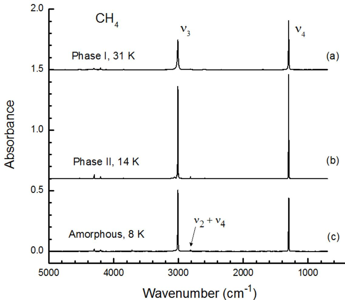
**Fig. 1** Infrared spectra of the three phases of solid CH<sub>4</sub> studied, each sample having a thickness of  $\sim 0.52 \mu\text{m}$ . See Chapados and Cabana<sup>6</sup> for expansions of the  $\nu_3$  and  $\nu_4$  regions of crystalline CH<sub>4</sub>, and Gerakines and Hudson<sup>9</sup> for the same for amorphous CH<sub>4</sub>. Spectra are offset for clarity.
