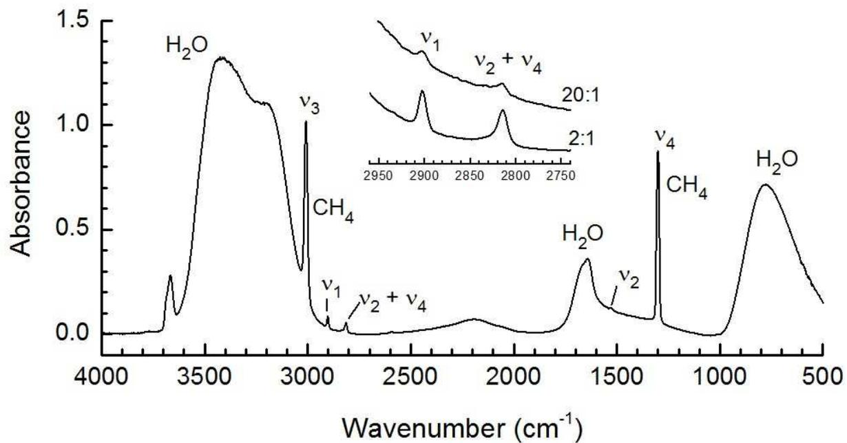
**Fig. 3** Infrared spectra of amorphous  $\text{H}_2\text{O} + \text{CH}_4$  (2:1) near 20 K showing the forbidden  $\nu_1$  and  $\nu_2$  bands taken in reflectance.<sup>19</sup> The inset shows the region around  $\nu_1$  for a more-dilute ice. The thicknesses for the (2:1) and (20:1) ices were about 4  $\mu\text{m}$ .
