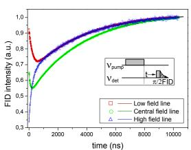
**Fig.4** Polarization Recovery (PR) curves and fits (solid lines) of the **FN-2a** FID for pumping on the high field line and detect at the same line (PR-EPR, blue triangles) or on one of the other hf lines (PR-ELDOR, green circles and red squares). Exp. conditions:  $c \sim 1.5$  mM,  $t_{\pi/2} = 24$  ns;  $t_{pump} = 0.1$  µs;  $B_1 \sim 2-3$  G; The length of the pump pulse is here shorter as steady state is not required. Inset: pulse sequence for PR-ELDOR and PR-EPR.
