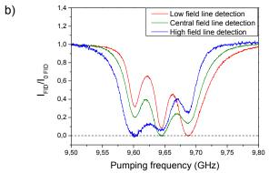
**Fig.3** Normalized FID intensity of TL (a) and **FN-2a** (b) as a function of the pumping ELDOR frequency. Experimental conditions:  $c \sim 1.5$  mM,  $t_{\pi/2} = 24$  ns;  $t_{pump} = 1$  µs;  $B_1 \sim 2-3$  G. The length of the pump pulse was adjusted to observed a complete saturation of the pumped line and to reach steady state. Inset: pulse sequence in the ELDOR saturation experiment.
