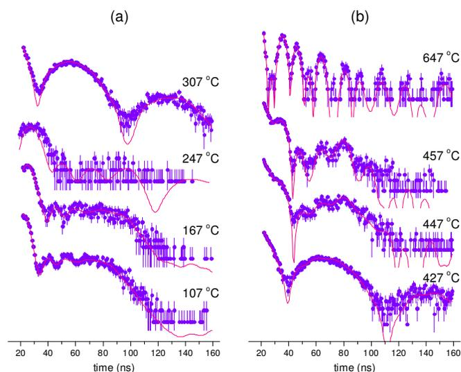
Fig. 11. Selected records obtained from NFS for the  $(\text{Fe}_{1-x}\text{Co}_x)_{76}\text{Mo}_8\text{Cu}_1\text{B}_{15}$  ( $x = 0.25$ ) at the indicated temperatures in the vicinity of  $T_C$  (a) and  $T_{x1}$  (b). Experimental data (symbols) are fitted (solid lines) according to the model described in the text.
