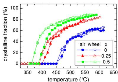
Fig. 6. Crystalline fraction plotted against the temperature of annealing as obtained from the deconvolution of *in situ* DSR data recorded from the air (full symbols) and the wheel (open symbols) sides of the  $(\text{Fe}_{1-x}\text{Co}_x)_{76}\text{Mo}_8\text{Cu}_1\text{B}_{15}$  alloy. Solid lines are only guide to the eye.
