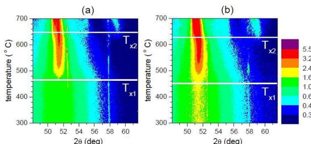
Fig. 2. Contour plots of diffractograms recorded by *in situ* DSR from the air (a) and the wheel (b) side of the  $(\text{Fe}_{1-x}\text{Co}_x)_{76}\text{Mo}_8\text{Cu}_1\text{B}_{15}$  ( $x=0$ ) alloy. Crystallization temperatures  $T_{x1}$  and  $T_{x2}$  are indicated by the horizontal white lines.
