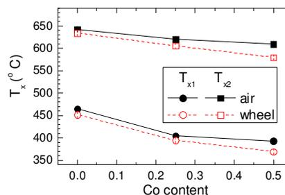
Fig. 5. Crystallization temperatures  $T_{x1}$  and  $T_{x2}$  plotted against the Co content in the  $(\text{Fe}_{1-x}\text{Co}_x)_{76}\text{Mo}_8\text{Cu}_1\text{B}_{15}$  alloys as derived from *in situ* DSR taken from both air and wheel sides of the ribbons. The lines are only guides to the eye.
