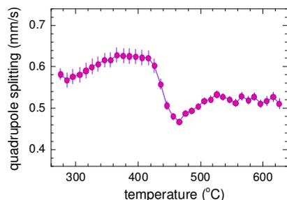
Fig. 14. Average values of quadrupole splitting of the amorphous residual matrix plotted against the annealing temperature as obtained from the fitting of *in situ* NFS data of the  $(\text{Fe}_{1-x}\text{Co}_x)_{76}\text{Mo}_8\text{Cu}_1\text{B}_{15}$  ( $x = 0.25$ ) alloy. Solid line is only guide to the eye.
