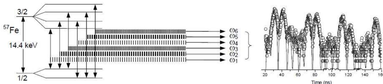
Fig. 1. Magnetically split nuclear levels of  $^{57}\text{Fe}$  (left), photons from de-excitation transitions that are characterized by the frequencies (energies)  $\omega_1$  to  $\omega_6$  (middle), and the resulting interferogram (right).
