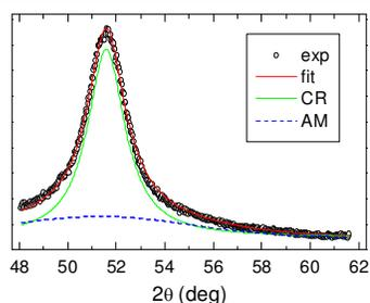
Fig. 7. Deconvolution of a diffractogram obtained from the wheel side of the  $(\text{Fe}_{1-x}\text{Co}_x)_{76}\text{Mo}_8\text{Cu}_1\text{B}_{15}$ ,  $x = 0.5$  alloy at 450 °C. The individual components correspond to the crystalline phase (CR) and to the residual amorphous matrix (AM).
