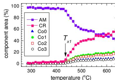
Fig. 12. Fraction of the residual amorphous matrix (AM) and bcc-(Fe,Co) crystalline phase (CR) plotted against the annealing temperature as obtained from the fitting of *in situ* NFS data of the  $(\text{Fe}_{1-x}\text{Co}_x)_{76}\text{Mo}_8\text{Cu}_1\text{B}_{15}$  ( $x = 0.25$ ) alloy. Fractions of crystalline sites with different amounts of Co nearest neighbours (Co0 – Co3) are also given. Solid lines are only guide to the eye. The arrow indicates the onset of crystallization  $T_{x1}$ .
