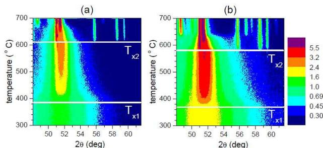
Fig. 4. Contour plots of diffractograms recorded by *in situ* DSR from the air (a) and the wheel (b) side of the  $(\text{Fe}_{1-x}\text{Co}_x)_{76}\text{Mo}_8\text{Cu}_1\text{B}_{15}$  ( $x=0.5$ ) alloy. Crystallization temperatures  $T_{x1}$  and  $T_{x2}$  are indicated by the horizontal white lines.
