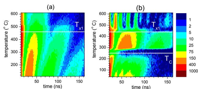
Fig. 10. Contour plot of 3-D nuclear forward scattering data of  $(\text{Fe}_{1-x}\text{Co}_x)_{76}\text{Mo}_8\text{Cu}_1\text{B}_{15}$  for  $x = 0$  (a) and  $x = 0.25$  (b). Crystallization  $T_{x1}$  and Curie  $T_C$  temperatures are indicated by the horizontal white lines.
