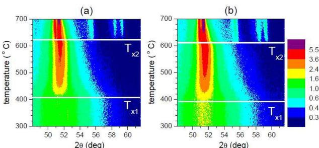
Fig. 3. Contour plots of diffractograms recorded by *in situ* DSR from the air (a) and the wheel (b) side of the  $(\text{Fe}_{1-x}\text{Co}_x)_{76}\text{Mo}_8\text{Cu}_1\text{B}_{15}$  ( $x=0.25$ ) alloy. Crystallization temperatures  $T_{x1}$  and  $T_{x2}$  are indicated by the horizontal white lines.
