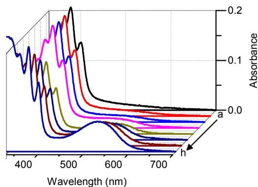
Fig. 3 Changes in the absorption spectra of DNA-bound **CP** by the addition of **EHD** in phosphate buffer (10 mM, 7.4) containing 2 mM NaCl. [**CP**], 16  $\mu\text{M}$ ; [**DNA**], 27  $\mu\text{M}$ ; [**EHD**], (a) 0 and (h) 15  $\mu\text{M}$ .
