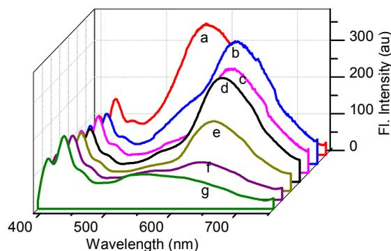
Fig. 2 Changes in the emission spectra of DNA-bound **CP** by the addition of **EHD** in phosphate buffer. [**CP**], 16  $\mu\text{M}$ ; [**DNA**], 27  $\mu\text{M}$ ; [**EHD**], (a) 0 and (g) 15  $\mu\text{M}$ . Excitation wavelength, 380 nm.
