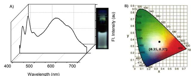
**Fig. 5** A) Emission spectrum of a solution containing **CP**, DNA and **PI** in the ratio 1:0.75:0.05 in aqueous medium. Excitation wavelength, 380 nm. Insets show the fluorescence of the same solution under UV lamp (365 nm). B) CIE Coordinates of the white light emission.
