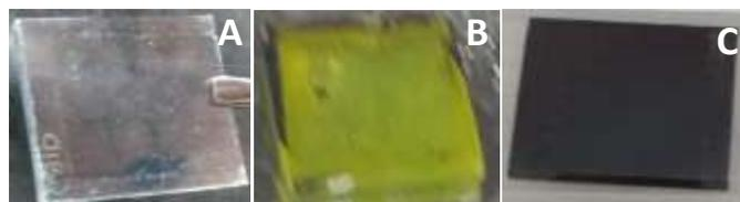
**Figure 1:** Colourless lead thiocyanate Pb(SCN)<sub>2</sub> film (A) Yellow intermediate film formed upon exposure to MAI vapours (B) and complete perovskite film (C)
