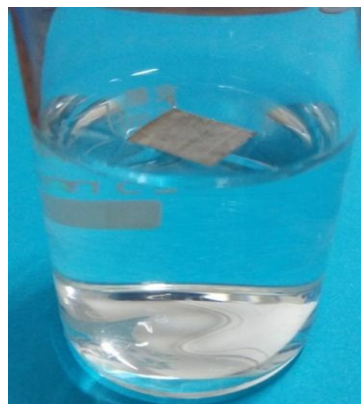
Fig. 10 Optical image of the superhydrophobic sample floating on the water.
