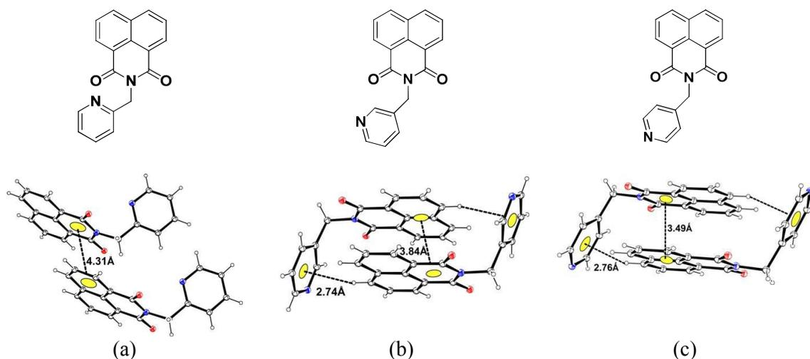
Figure 15: Three positional isomers of N-(pyridylmethyl)-1,8-naphthalimide and their respective self-assemblies.
