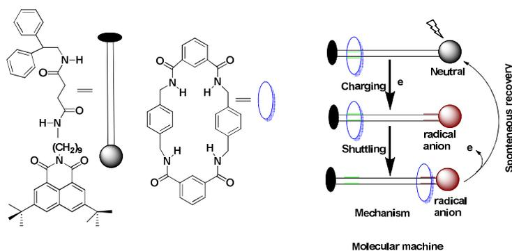
Scheme 8: A molecular machine based on naphthalimide derivatives
