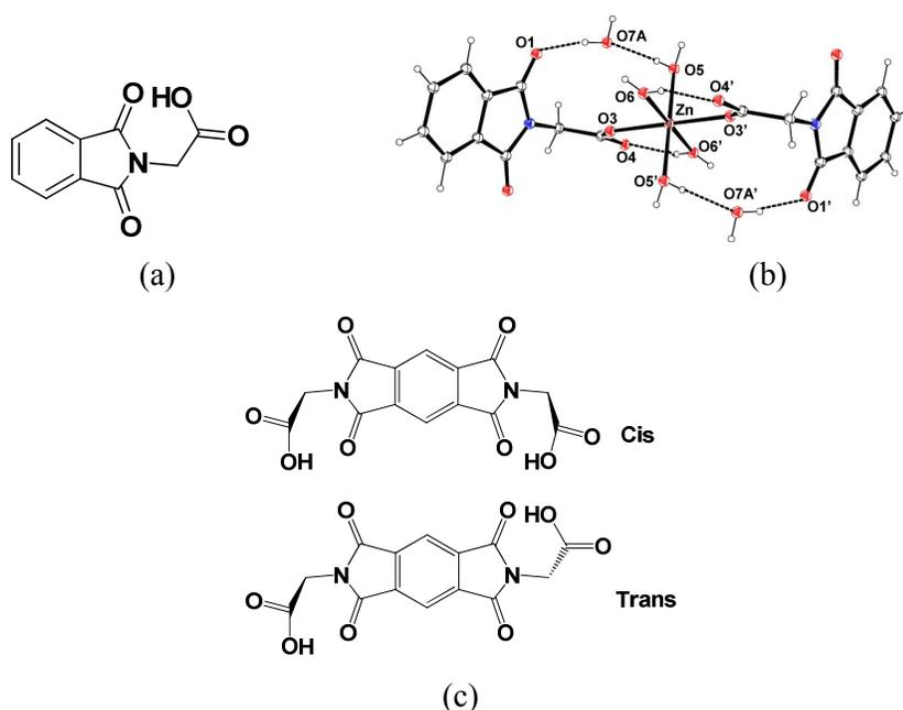
Figure 14: (a) Structure of N-phthaloylglycine, (b) Structure of tetra-aqua-bis-N-phthaloylglycinato zinc (II) dihydrate (c) Cis and trans rotamers of N,N'-bis(glycinyl)pyromellitic diimide.
