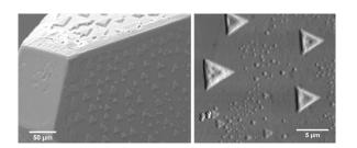
Sylvite crystals are grown from solution in the presence of lead. An epitaxial model explains both habit and surface modifications.
