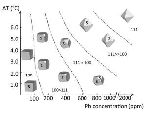
**Figure 1.** Morphodrome of KCI crystals growing at different supersaturation values and under different Pb concentration (ppm) in solution; label *s* indicates the presence of growth spirals on the growing faces. Inspired and elaborated from reference 10. See S.I., Fig. 1 for details.
