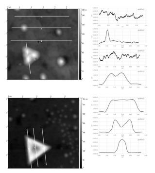
**Figure 5**. Early stages of the patterns observed on the {111} KCl form grown in the presence of Pb ions (AFM pictures). Single and triple KCl hillocks emerging on a rough surface (top left). The corresponding profiles are referred to a single hillock and to the averaged thickness (15 nm) of the rough surface (top right). A triple hillock (bottom left) shows a complex morphology, as follows from the profiles obtained from three different and parallel cuts (bottom right).
