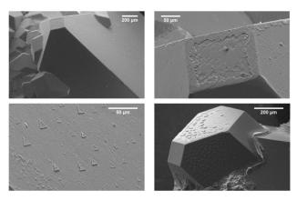
**Figure 4.** SEM images of KCl crystals grown from Pb doped solutions. The octahedron dominates the cube (top-left). The surface growth pattern of a cube face is made by layers running parallel to the diagonals of the face, i.e. by <100> macrosteps (top-right). Trigonal 3D islands nucleate on the octahedron faces: the filling up of the islands starts from their periphery (bottom-left). Islands, once completely filled, show their terraces parallel to the {111} substrate (bottom-right).
