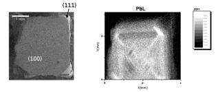
**Figure 2**. The SEM image of the sample, used as a morphological reference for the Pb distribution inside the crystal (left side). Pb concentration, in ppm (right side).
