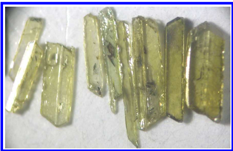
Optical images of strip-shape diamond crystals grown by a floatage system with FeCr acted as solvent-metal
