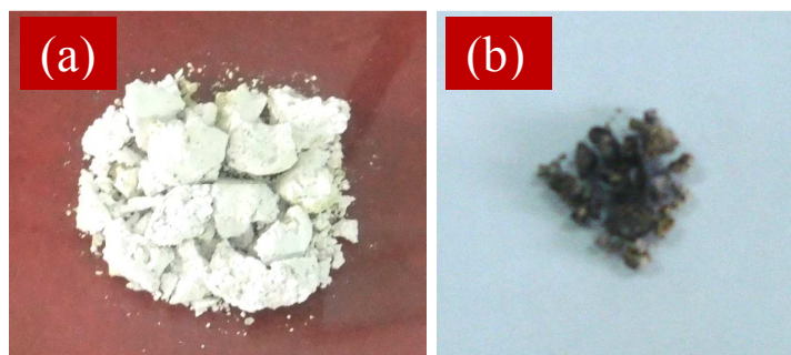
Fig. 8 Digital images of the dried-gel material (a) just before the adsorption and (b) after completion/saturation of the adsorption process indicating the continuous uptake of molecular iodine by the gel matrix from solution phase.
