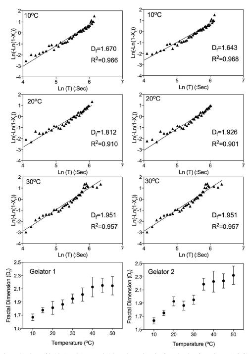
Figure 9. Plots of  $\ln(-\ln(1-Xr))$  versus  $\ln(T)$  to determine the fractal value for gelators 1 (left) and 2 (right) at 10, 20 and 30 °C. Synopses of the fractal values versus crystallization temperature are also shown at the bottom.
