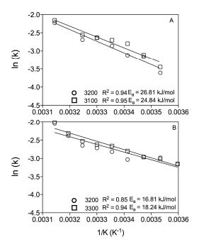
Figure 8. Calculation of the activation energy from an Arrhenius plot of the rate constants from the Avrami equation while n = 2 for 1 (A) and 2 (B) in mineral oil.
