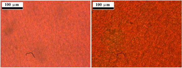
Figure 4. Polarizing optical micrographs at 23 °C of a 2 wt % 1 in mineral oil gel prepared by the fast- (left) and slow-cooling (right) protocols.
