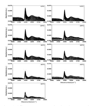
Figure 2. Offset FT-IR spectra, using the sol spectra as the baselines, for formation of 2 wt % mineral oil gels of 1 at different temperatures.
