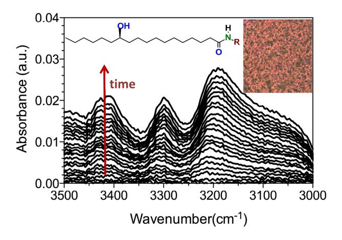
Infra-red synchrotron radiation is used to monitor the formation of fibrillar networks as sols of simple gelators become gels.
