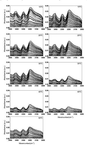
Figure 5. Offset FT-IR spectra, using the sol spectra as the baselines, for formation of mineral oil gels of 2 at different temperatures.
