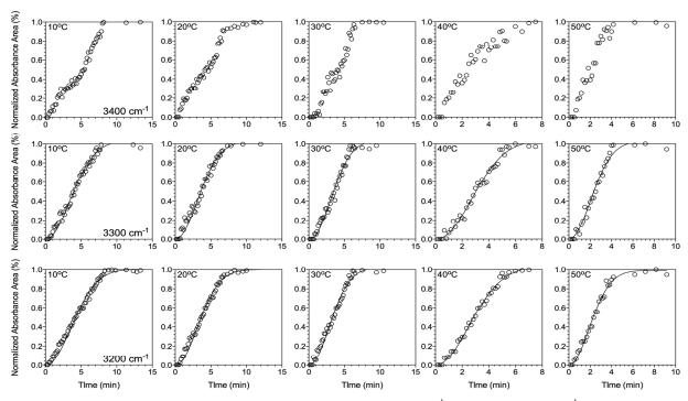
Figure 6. Integrated and normalized data for the peak areas at 3400 cm<sup>-1</sup> (top row), 3300 cm<sup>-1</sup> (middle row) and 3200 cm<sup>-1</sup> (bottom row) for the mineral oil gels of compound 2 at each of the isothermal crystallization temperatures.
