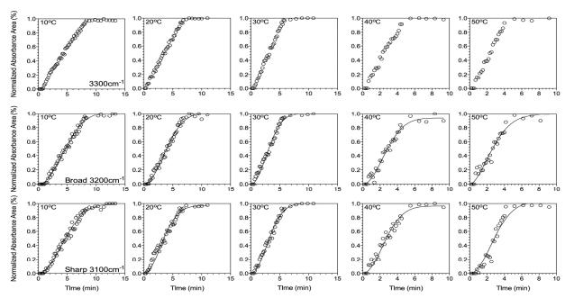
Figure 3. Integrated and normalized data for the areas of the sharp peaks at 3300 cm<sup>-1</sup> (top row), the broad peaks between 3050 and 3250 cm<sup>-1</sup> and the weak peaks between 3150 and 3250 cm<sup>-1</sup> for samples of 1 in the mineral oil at different isothermal crystallization temperatures.
