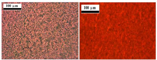
Figure 7. Polarizing optical micrograph at 23 °C of a 2 wt % 2 in mineral oil gel prepared by the fast- (left) and slow-cooling (right) protocols.
