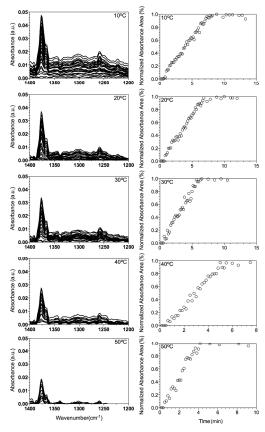
Figure 1. Vertically offset FT-IR spectra for the aliphatic CH<sub>3</sub> stretch, using the sol spectra as the baseline, for formation of 2 wt % mineral oil gels of 1 at different temperatures (left). The peak areas at 1375 cm<sup>-1</sup> were integrated and normalized by dividing the values by the maximum absorbance area obtained after holding the gel for 5 min at the crystallization temperature (right).
