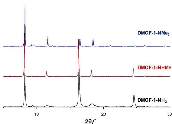
**Figure 1** PXRD patterns and <sup>1</sup>H NMR spectra of DMOF-1-NH<sub>2</sub>, -NHMe and -NMe<sub>2</sub>.
