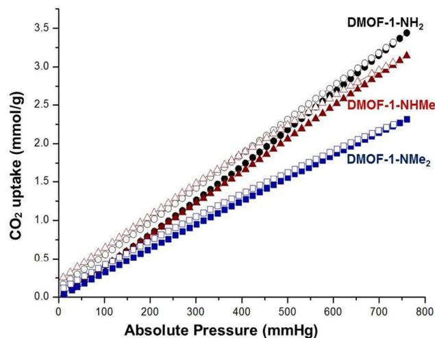
Figure 4 CO<sub>2</sub> isotherms (298 K) of DMOF-1-NH<sub>2</sub> (circle, black), -NHMe (triangle, red) and -NMe<sub>2</sub> (square, blue). Adsorption and desorption traces are indicated by filled and open symbols, respectively.
