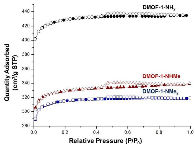
Figure 3 N<sub>2</sub> isotherms (77 K) of DMOF-1-NH<sub>2</sub> (circle, black), -NHMe (triangle, red) and -NMe<sub>2</sub> (square, blue). Adsorption and desorption traces are indicated by filled and open symbols, respectively.
