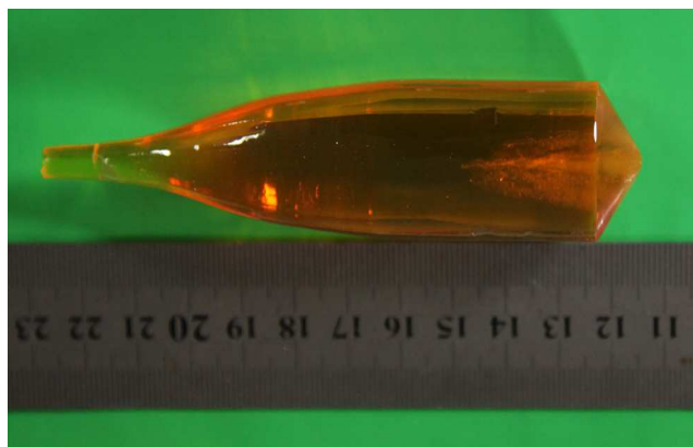
Fig.1 As-grown Ce,Mn:YAG single crystal grown by Czochralski
