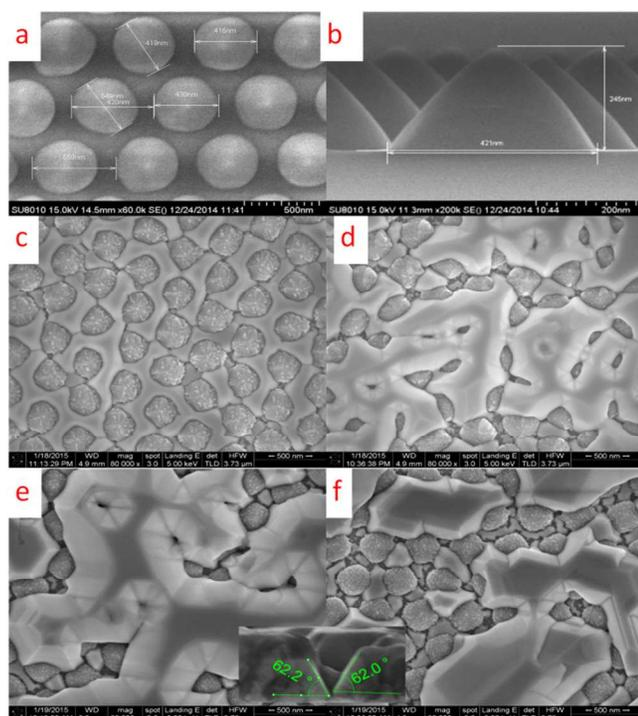
Fig. 4 SEM images of the cone-shape NPSS with (a) bird view and (b) side view, and GaN 3D growth behaviors for (c) 100 (d) 300 (e) 600 and (f) 800 s, respectively. The inset shows the cross-sectional SEM image of the typical pattern for (e) and (f)
