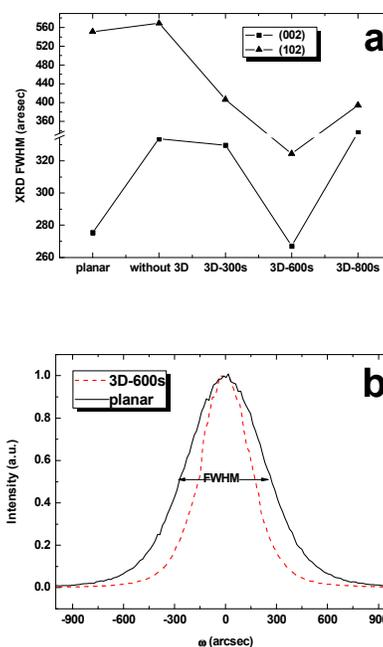
Fig. 1 (a) the dependence of XRD FWHM of GaN films on different 3D growth time for on planar sapphire and NPSS. (b) XRD rocking curves of (102) plane for planar samples and NPSS with 3D growth time for 600 s.
