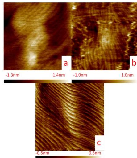
Fig. 3 AFM images of GaN films grown on (a) the planar sapphire substrate (b) the NPSS without 3D growth and (c) the NPSS with 3D growth. All topographic AFM images are scaled in  $3\text{ }\mu\text{m} \times 3\text{ }\mu\text{m}$ .
