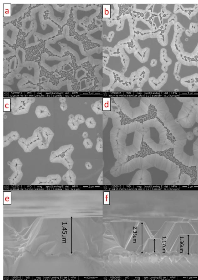
Fig.5 SEM images of GaN recovery growth for a) 300, b) 600, c) 1200 s on the templates with 600s 3D growth, and d) 1200s on the template with 800 s 3D growth model; (e) and (f) were cross-sectional images of 1200s on the template with 600 and 800 s 3D growth stage.
