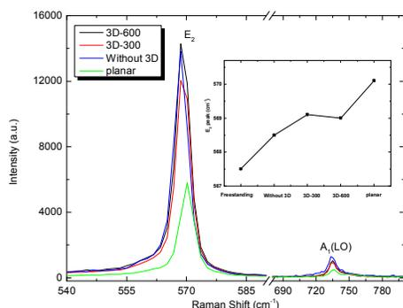
Fig.2 Raman spectra of GaN films grown on planar sapphire and NPSS with different 3D growth time. The inset is  $E_2$  peaks for different GaN films fitting by Gaussian function, the start point is for the freestanding GaN which is free of strain.
