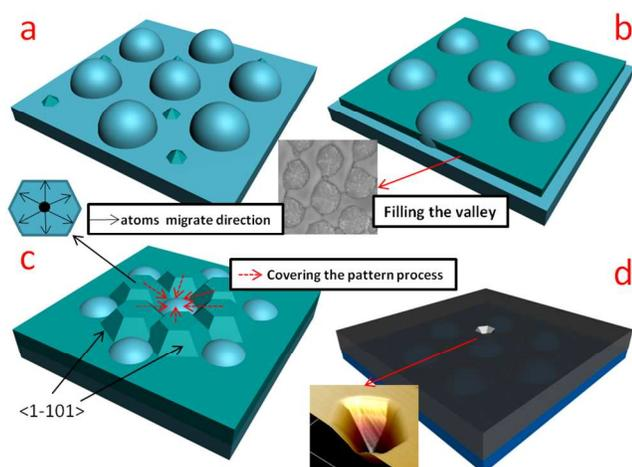
Fig. 6 Schematic drawing of the two-step growth mode procedure of GaN epitaxy on the NPSS. (a) Buffer layer and nucleation, (b) 3D growth, (c) 3D growth and recovery growth, (d) recovery growth.
