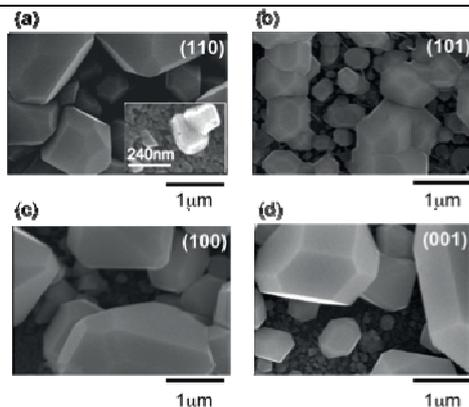
Figure 7. SEM images of  $\text{Ag}_7\text{O}_8\text{HSO}_4$  crystals that were used in the XRD analysis shown in Fig. 6.
