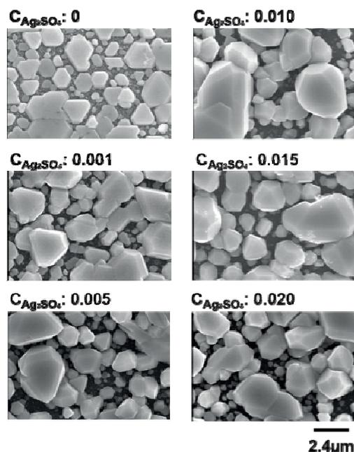
Figure 8. A series of SEM images of silver oxide clathrate compounds photodeposited in solutions of  $\text{AgNO}_3$  and  $\text{Ag}_2\text{SO}_4$  with different mixing ratios at an electrode potential of +0.3V vs Ag in 1 h.
