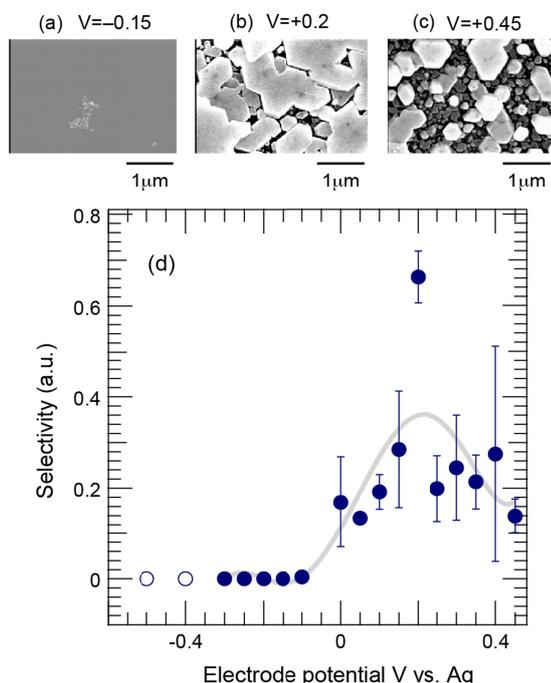
Figure 5. Relative selectivity of the formation of Ag<sub>7</sub>O<sub>8</sub>NO<sub>3</sub> (filled circles) as a function of electrode potential, together with SEM images taken for samples grown at electrode potentials of -0.15, +0.2 and +0.45V, respectively. Open circles correspond to the formation of Ag metal particles.
