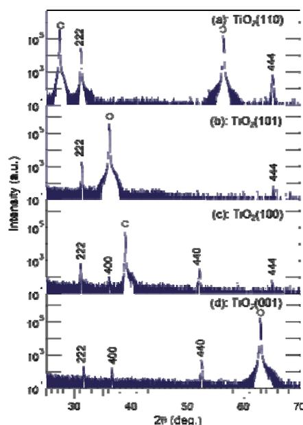
Figure 1. A set of  $\theta$ - $2\theta$  XRD patterns of photoelectrochemically deposited  $\text{Ag}_7\text{O}_8\text{NO}_3$  on Nb-doped  $\text{TiO}_2(110)$ , (101), (100), and (001) single-crystal substrates in a 0.01M  $\text{AgNO}_3$  solution at an electrode potential of  $+0.3$  V vs Ag. The deposition time was 2 h. All plots are shown on a logarithmic scale.
