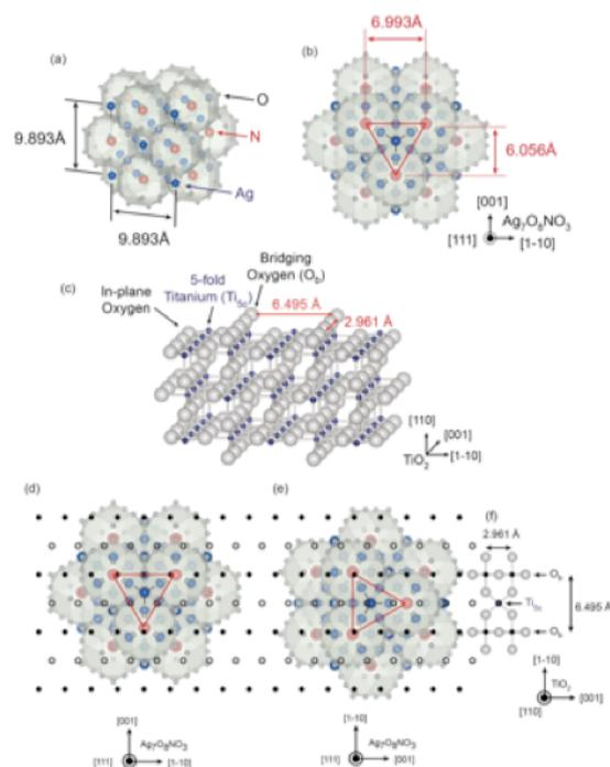
Figure 4. (a) Schematic illustration of the  $\text{Ag}_7\text{O}_8\text{NO}_3$  crystal structure in a cubic system. Blue, red, and gray spheres denote Ag, N, and O, respectively. (b) A view of the (111) surface of a  $\text{Ag}_7\text{O}_8\text{NO}_3$  crystal.
