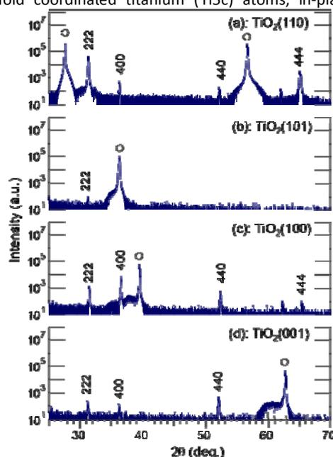
Figure 6. A set of  $\theta - 2\theta$  XRD patterns of photoelectrochemically deposited Ag<sub>7</sub>O<sub>8</sub>HSO<sub>4</sub> samples grown on (110), (101), (100), and (001) oriented Nb-doped TiO<sub>2</sub> substrates. These crystals were grown in a 0.01M Ag<sub>7</sub>O<sub>8</sub>HSO<sub>4</sub> solution at an electrode potential of +0.3V vs Ag in 2 h. All plots are shown on a logarithmic scale.
