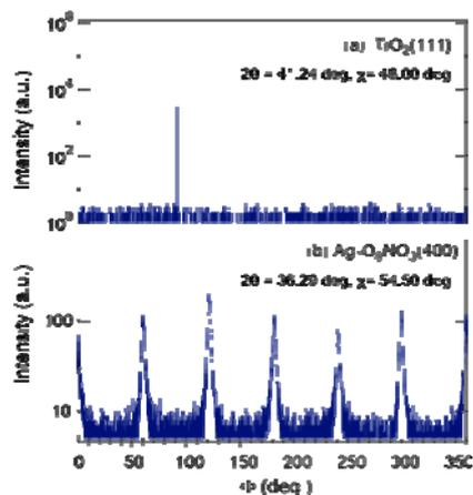
Figure 3. X-ray  $\Phi$  scans of the  $\text{TiO}_2(111)$  and  $\text{Ag}_7\text{O}_8\text{NO}_3(400)$  reflections for a (111)-oriented  $\text{Ag}_7\text{O}_8\text{NO}_3$  sample epitaxially grown on a  $\text{TiO}_2(110)$  substrate. Six clathrate peaks were observed from two equivalent domains rotated by  $180^\circ$  relative to each other.
