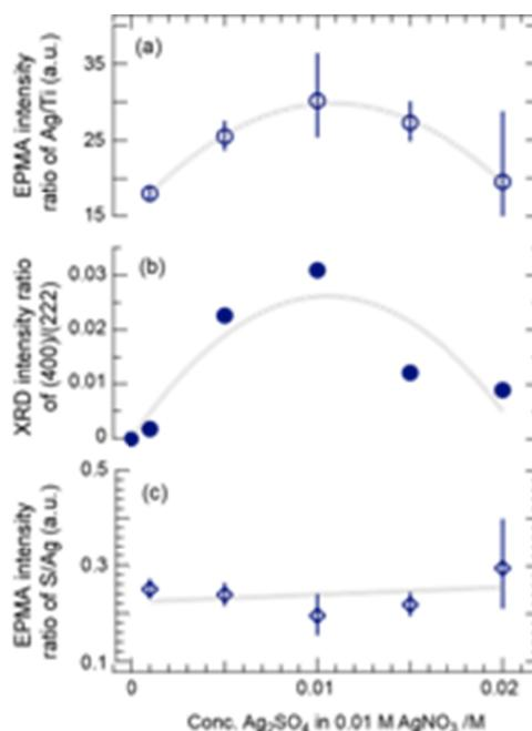
Figure 9. (a) EPMA intensity ratio of Ag/Ti as a function of the  $\text{Ag}_2\text{SO}_4$  concentration in the photodeposition solution. The Ag/Ti ratio is proportional to the total amount of photodeposited silver oxide clathrate compounds. (b) Intensity ratio of the (400) and (222) XRD peaks. (c) EPMA S/Ag intensity ratio as a function of  $C_{\text{Ag}_2\text{SO}_4}$ .
