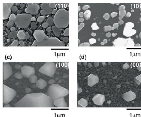
Figure 2. SEM images of the same set of  $\text{Ag}_7\text{O}_8\text{NO}_3$  samples that were used for the XRD analysis in Fig. 1.
