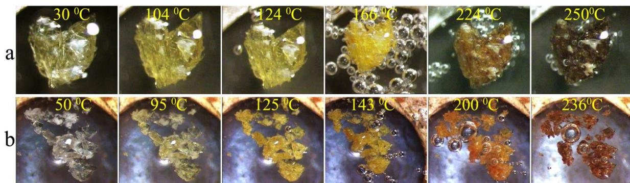
**Figure 7.** Hot stage microscope photograph of compounds **1** (a) and **2** (b) to showing the release of solvent at various temperatures. The crystals were immersed in silicone oil to indicate the release of solvent molecules.
