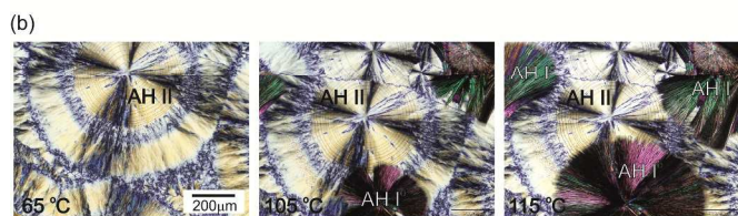
Fig. 6 (a) DSC curves (heating rate 10 °C \text{min}^{-1} ) of 4-AQ anhydrate polymorphs; mp – melting point. The inserts show the glass transition and AH II \rightarrow AH I o phase transformation. (b) Microphotographs showing the AH II \rightarrow AH I o phase transformation in the temperature range 105 to 115 °C.
