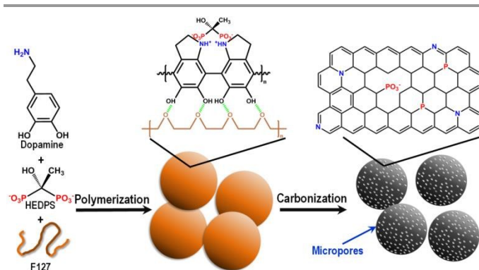
Fig. 1 Schematic synthesis process of N,P-codoped microporous carbon spheres.
