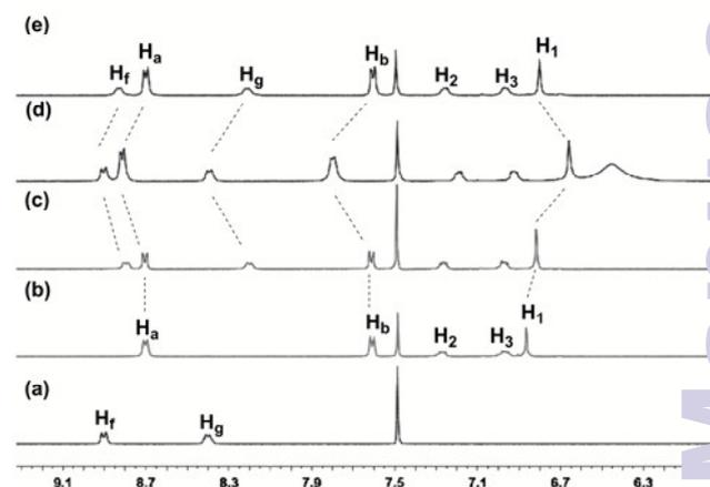
**Fig. 6** Partial <sup>1</sup>H NMR spectra (300 MHz, CD<sub>3</sub>CN/CDCl<sub>3</sub> = 1:1, 298 K) of (a) free **6**, (b) **1** and 1.0 equiv of 4,4'-bipyridine, (c) to the solution of b was added 1.0 equiv. of **6**, (d) to the solution of c was added 4.0 equiv. of TFA, and (e) to the solution of c was added 6.0 equiv. of Et<sub>3</sub>N. [**1**]<sub>0</sub> = 3.0 mM.
