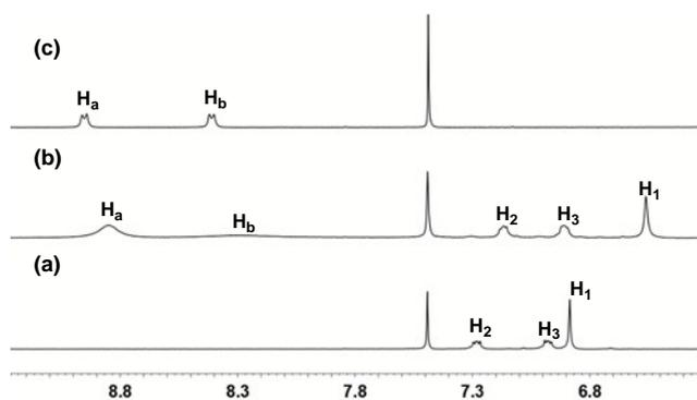
**Fig. 2** Partial  $^1\text{H}$  NMR spectra (300 MHz, 298 K,  $\text{CD}_3\text{CN}/\text{CDCl}_3 = 1:1$ , v/v) of (a) free **1**, (b) **1** and 1.0 equiv of **2**, (c) free **2**.  $[\mathbf{1}]_0 = 3.0$  mM.
