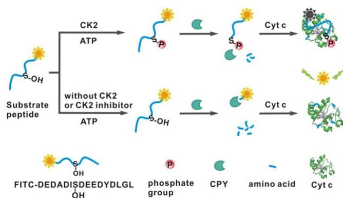
**Scheme 1** Schematic illustration of the Cyt c-peptide sensing platform for the detection of CK2 activity and inhibition based on phosphorylation against CPY degradation.
