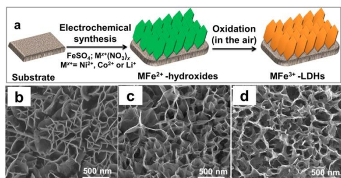
Figure 2. (a) Schematic illustration for the synthetic route of MFe-LDH ( \text{M} = \text{Co}, \text{Ni} and \text{Li} ) nanoarrays. SEM images of (b) NiFe-LDH, (c) CoFe-LDH and (d) LiFe-LDH nanoplatelet arrays, respectively. Reproduced with permission from ref. 46.
