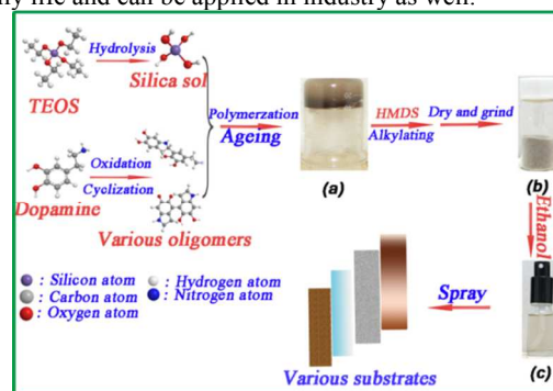
Figure 1. Schematic illustration of the synthesis procedure of DSTM gel nanocoating. Optical photographs of (a) DOPA-silica gel. (b) DSTM gel powder. (c) DSTM gel nanocoating.
