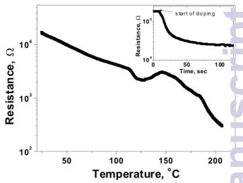
Fig. 3 (a) Temperature dependence of the resistance for a doped CuCl<sub>2</sub> xerogel 1 during the annealing (main panel). Top inset shows typical dependence of resistance vs time during doping by iodine vapor at room temperature.
