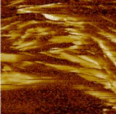
**Fig. 4** Topography (top) and current (bottom, bias voltage 1.1 V) images from C<sup>c</sup> AFM of the same region (3×3 microns) of a CuCl<sub>2</sub> xerogel of **1** on highly oriented pyrolytic graphite. The brighter regions in the current map correspond to high conductivity. The independence of the responses is highlighted by the insulative bump in the topographic image.
