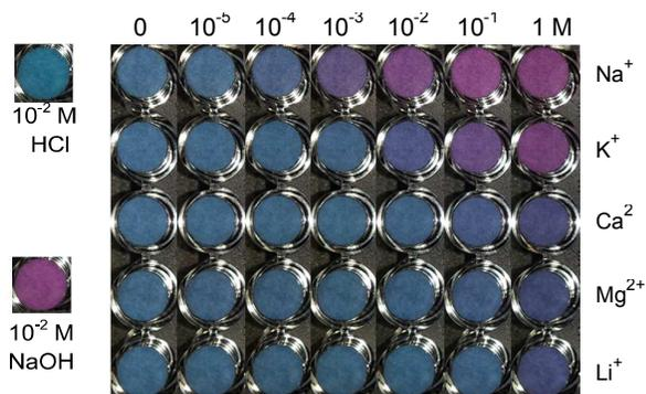
Fig. 1 Pictures of one paper-based  $\text{Na}^+$ -selective optode in  $10^{-2}$  M HCl and NaOH solution, respectively, and five optodes (from top to bottom) in pH 7.4 Tris-HCl buffer containing increasing concentrations of NaCl, KCl,  $\text{CaCl}_2$ ,  $\text{MgCl}_2$ , and LiCl, respectively.
