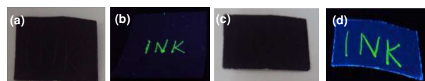
Figure 6. (a) The word INK (from compound D2) written by an injector (a & c) under visible light illumination, (b & d) under UV light illumination.
