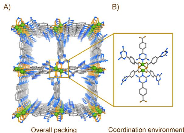
**Figure 2:** a) Perspective view of the overall packing of DAT-MOF-1a (guest molecules and H atoms are omitted for clarity); b) Lewis basic N-rich  $\pi$ -electron deficient coordination environment constructing DAT-MOF-1a, rendering the channel functionalization.
