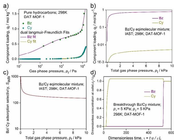
**Figure 4:** a) Comparison of experimental data for pure component isotherms for Bz and Cy in DAT-MOF-1 with dual-Langmuir-Freundlich fits that are shown by the continuous solid lines; b) IAST calculations for Bz uptake capacity for equimolar Bz/Cy mixtures in DAT-MOF-1; c) IAST calculations of adsorption selectivity for equimolar mixtures for equimolar Bz/Cy in DAT-MOF-1; d) Breakthrough simulations for Bz/Cy in fixed bed of DAT-MOF-1 at 298 K.
