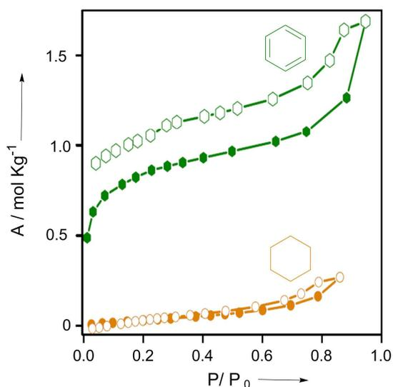
**Figure 3:** Solvent sorption isotherms for compound DAT-MOF-1 recorded at 298 K for Bz and Cy. Closed and open symbols denote adsorption and desorption, respectively.
