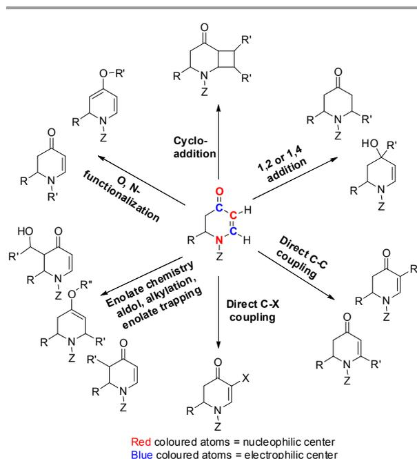
Figure 2: Reactive sites and possible transformations of cyclic enamines.
