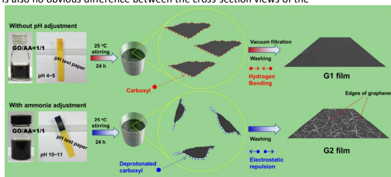
Fig. 1 Schematic illustration of the preparation procedures for carbocatalyst films G1 and G2.
