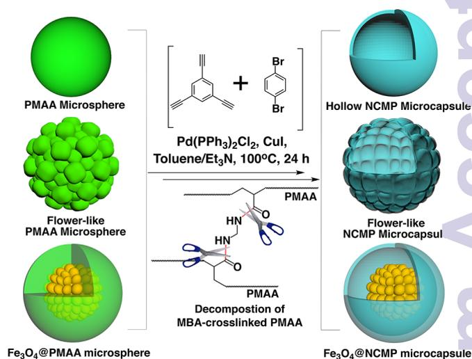
**Scheme 1.** Illustration of the modulation of NCMP nanostructures by using the various PMAA microspheres as self-sacrificial templates.
