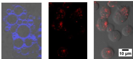
**Fig. 5** Left: Incorporation of **1** in GUVs at basic pH, images are the overlap of bright field and fluorescence ( $\lambda_{\text{ex}} = 405$  nm) detections to compare the membrane and chromophore localisations. Middle and right: Two-photon imaging of COS7 cells (middle) incubated with  $1\mu\text{M}$  of for **1** ( $\lambda_{\text{ex}} = 700$  nm) and overlap of bright field (right).
