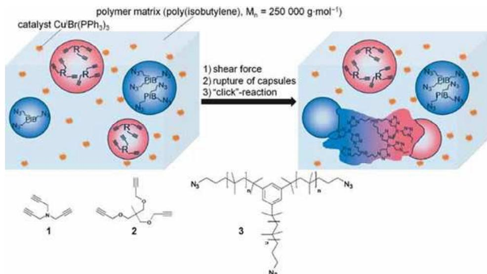
**Figure 14.** Design and extrinsic self-healing of polyisobutylene matrix embedded with microcapsules of small molecular weight alkynes and three-arm star polyisobutylene azides separately via azide-alkyne click reaction in the presence of Cu(I) species.<sup>132</sup> Copyright 2011 Wiley Interfaces.
