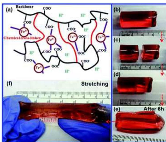
**Figure 10.** Schematic illustration of ionically-crosslinked hydrogels of poly(acrylic acids) with ferric ions (a) and digital images showing the occurrence of autonomous self-healing through dynamic bonding of physical crosslinking (b-f).<sup>99</sup> Copyright 2013 Royal Society of Chemistry.
