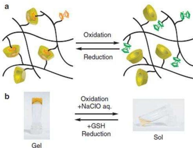
**Figure 11.** Schematic illustration of host-guest interactions between PAA-CD and PAA-Fc to form self-healable supramolecular hydrogels (a) and their digital images showing gel-sol transition.<sup>112</sup> Copyright 2011 Nature Publishing Group.
