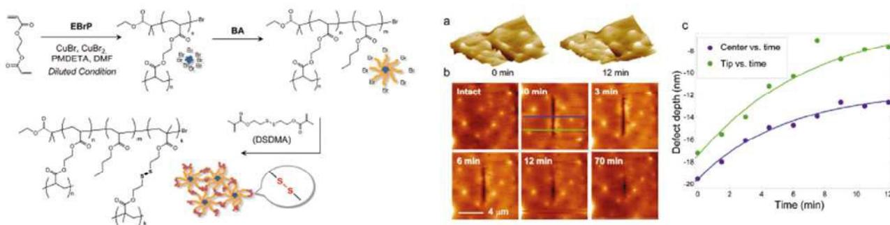
**Figure 2.** Chemical structure of disulfide-crosslinked star-shaped copolymer (left) and time dependent change of height mode AFM image for cut on the surface of reversibly disulfide-crosslinked star-polymer network (right): 3D images (a), 2D height mode images (b), and evolution of damage depth for 12 min at two positions (c).<sup>33</sup> Copyright 2012 American Chemical Society.
