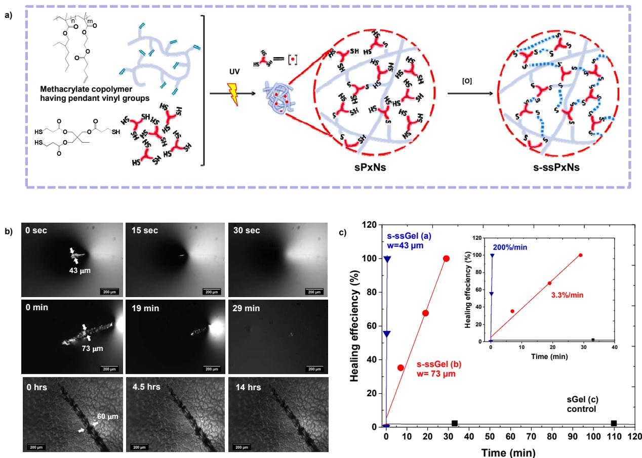
**Figure 3.** Illustration of a novel method utilizing click-type photo-induced thiol-ene radical addition and oxidation to synthesize dual sulfide-disulfide crosslinked networks (s-ssPxNs) (a), evolution of microscope images (b) and kinetics of self-healing (c) over time at room temperature for dual s-ssPxN with different cut sizes of 43 μm wide (upper) and 73 μm wide (middle), compared with a control of sPxN with no disulfide (bottom). Copyright 2015 Wiley Interfaces.
