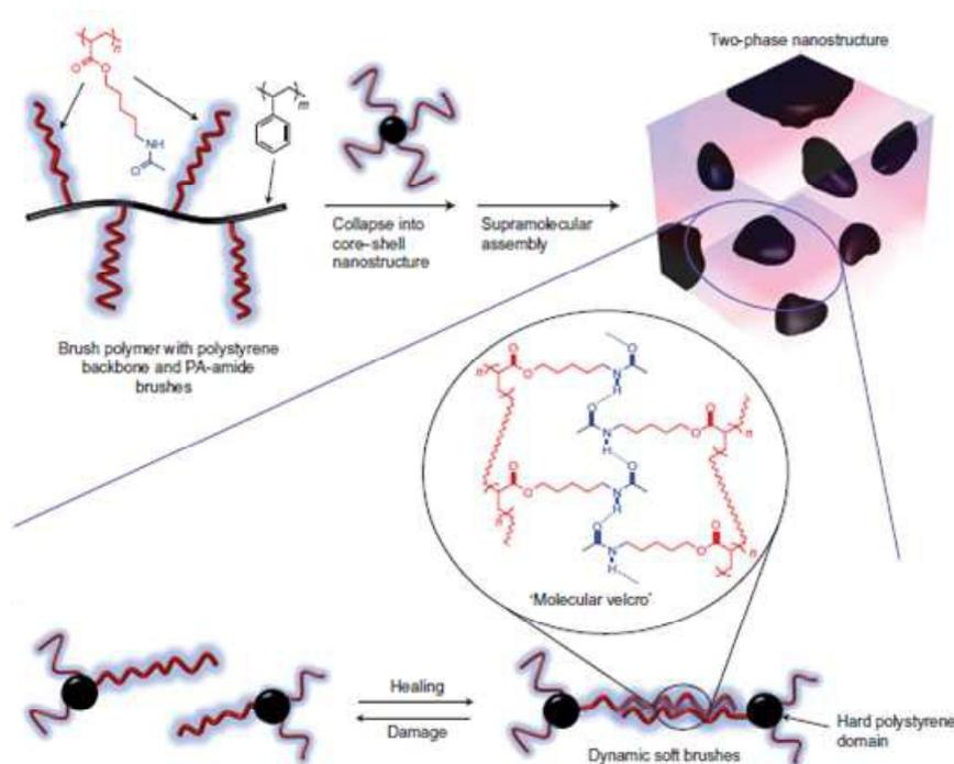
**Figure 7.** Schematic illustration of hydrogen-bonding brush polymer consisting of polystyrene backbone (high  $T_g$ ) as a hard phase and polyacrylate amide brushes (low  $T_g$ ) as a soft phase and its supramolecular assembly to form two-phase microstructures, consisting of hard polystyrene domains microphase-separated in soft matrix containing secondary amide groups that are capable of forming dynamic supramolecular networks.<sup>76</sup> Copyright 2014 Nature Publishing Group.
