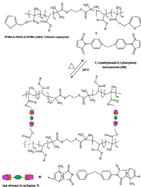
**Figure 5.** Schematic illustration of DA and retro-DA reaction occurred in reactive mixtures consisting of a ABA triblock copolymer having pendant furfuryl groups with 1,1'-(methylenedi-4,1-phenylene)bismaleimide for thermally-driven self-healing.<sup>46</sup> Copyright 2010 American Chemical Society.
