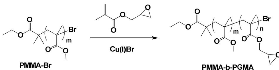
**Figure 13.** Illustration of ATRP of GMA from PMMA-Br macroinitiator for microcapsule-based extrinsic self-healing.
