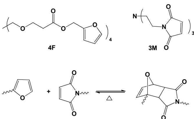
**Figure 4.** Illustration of polyaddition through DA reaction of a four-arm furan-labeled monomer (4F) and a three-arm maleimide-labeled monomer (3M) to form DA-crosslinked materials.<sup>37</sup>
