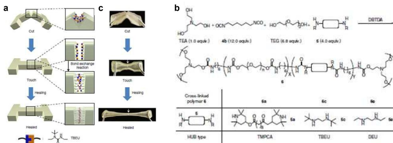
**Figure 6.** Schematic illustration of self-healing process (a), chemical structures and ratios of components used for the synthesis (b), and selected snapshots during the course of self-healing experiments of HUB-based crosslinked poly(urethane-urea) materials (c). TMPCA: 2,2,6,6-tetramethylpiperidinyloxy, TBEU: 1-(t-butyl)-1-ethylurea, and DEU: 1,1-diethylurea.<sup>54</sup> Copyright 2014 Nature Publishing Group.
