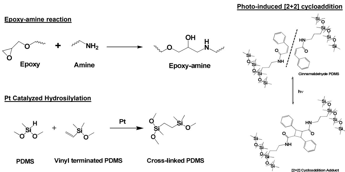
**Figure 15.** Illustration of various polyaddition mechanisms for the development of novel extrinsic self-healing materials.
