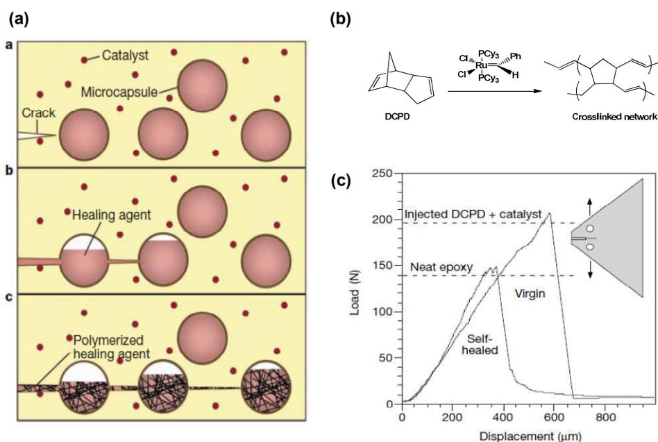
**Figure 12.** Pictorial depiction of healing mechanism of urea-formaldehyde microcapsule (a), healing chemistry utilizing ROMP of DCPD in the presence of Grubb's catalyst (b), and healing efficiency is obtained by fracture toughness testing of tapered double-cantilever beam (TDCB) specimens (c).<sup>120</sup> Copyright 2001 Nature Publishing Group.
