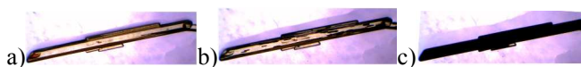
Figure 3: Observation of a single crystal of \text{CH}_3\text{NH}_3\text{PbI}_3\cdot\text{H}_2\text{O} ( 2 ) immersed in paratone oil at 298K in air and the spontaneous conversion to \text{CH}_3\text{NH}_3\text{PbI}_3 perovskite ( 1 ) recorded at different times a) t = 4 minutes b) t = 48 minutes c) t = 104 minutes.
