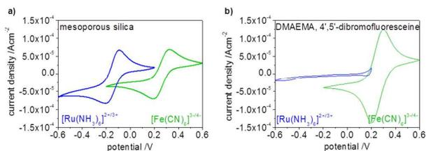
**Figure 5:** Cyclic voltammetry (25 mV/s) results at an acidic pH (2-3) clearly show the influence of the polymer (here DMAEMA) on ionic permselectivity (b) for a positively charged probe molecule ( $[\text{Ru}(\text{NH}_3)_6]^{2+/3+}$  blue) and a negatively charged probe molecule ( $[\text{Fe}(\text{CN})_6]^{3-/4-}$  green) in comparison to unmodified mesoporous silica (a).
