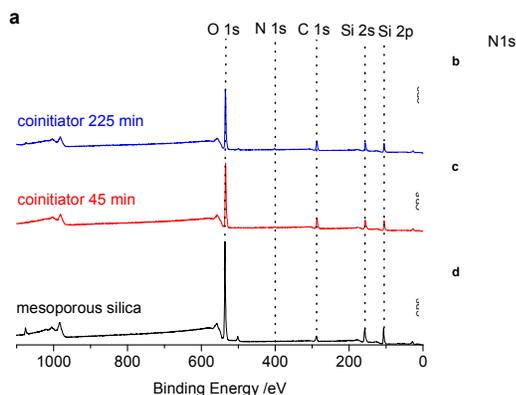
**Figure 3:** XP-spectra showing the co-initiator presence after functionalization for 45 minutes (red) and 225 minutes (blue) in comparison to non-functionalized mesoporous thin films (black) including the respective zoom into the N1s signal for the untreated mesoporous silica film (d) as well as after functionalization for 45 minutes (c) and 225 minutes (b).
