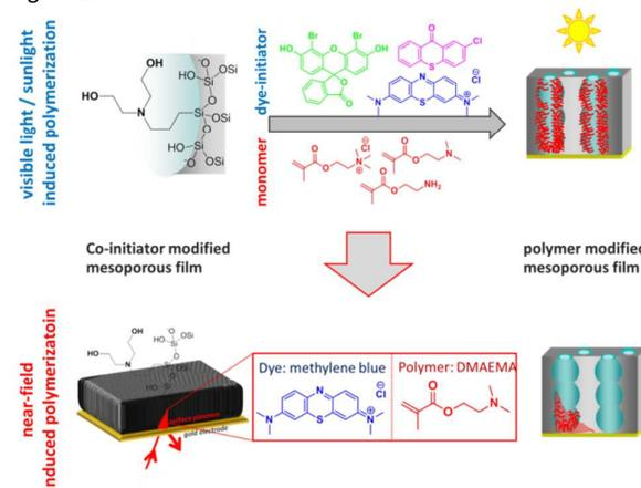
**Figure 1:** Schematic presentation of the visible light, sunlight, or surface plasmon near-field induced surface polymer modification of mesoporous thin silica films using dye-sensitized polymerizations.
