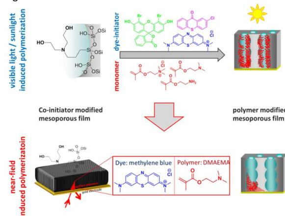
**Figure 1:** Schematic presentation of the visible light, sunlight, or surface plasmon near-field induced surface polymer modification of mesoporous thin silica films using dye-sensitized polymerizations.
