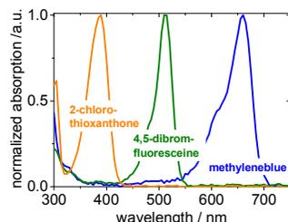
**Figure 2:** UV-Vis spectra of the applied dye initiators 2-chlorothioxanthone (orange), 4,5-dibromfluoresceine (green), and methylene blue (blue) measured in a water-based solution.
