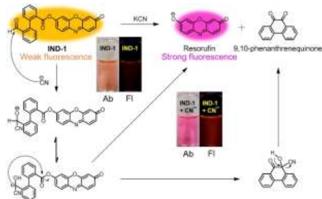
Scheme 2 KCN catalyzed intramolecular crossed-benzoin reaction of IND-1 .
