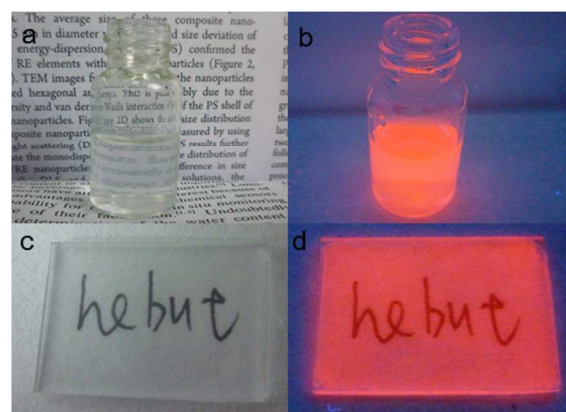
Fig. 3 Digital photographs of Eu 3+ (TTA) n @Lap dispersed in deionized water under (a) daylight and (b) UV illumination at 365 nm. Images of transparent thin film under (c) daylight and (d) the film under 365 nm UV irradiation.
