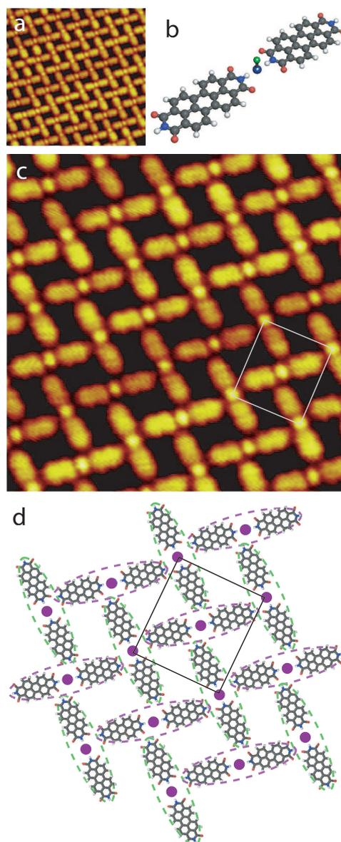
**Fig. 2** STM image of the PTCDI-NaCl nanoarchitecture after deposition on Au(111)- $(22 \times \sqrt{3})$  at room temperature and post annealing at 100 °C,  $V_s = 2.0$  V,  $I_t = 0.2$  nA; (a)  $15 \times 15$  nm<sup>2</sup>, (c)  $10 \times 10$  nm<sup>2</sup>. (b) Scheme of PTCDI·NaCl·PTCDI stick (perspective). (d) Model of the Mesh-nanoarchitecture. NaCl dipoles are represented by purple circles.
