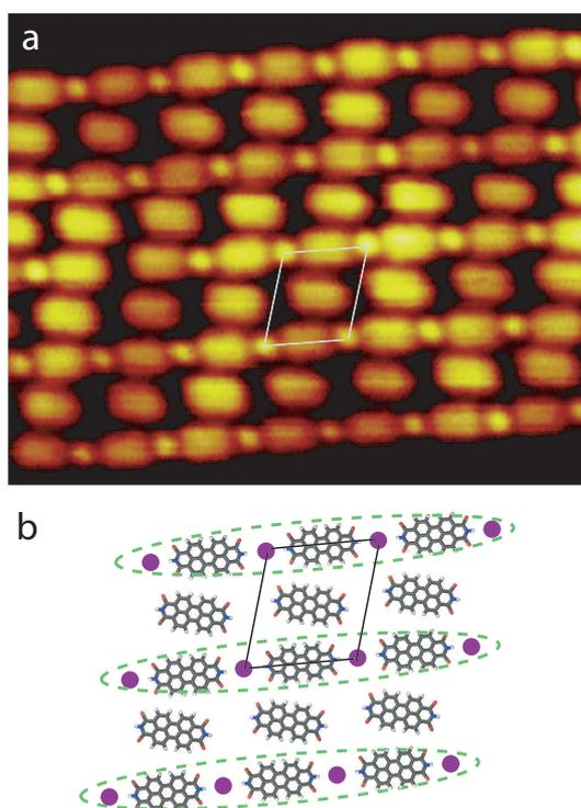
**Fig. 3** (a) STM image of the PTCDI-NaCl nanoarchitecture after deposition on Au(111)-(22  $\times$   $\sqrt{3}$ ) at room temperature and post annealing at 150  $^\circ$ C, 10  $\times$  8 nm $^2$ ;  $V_s = 1.9$  V,  $I_t = 0.2$  nA. (b) Model of the chain-nanoarchitecture. NaCl dipoles are represented by purple circles.
