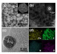
**Fig. 1** Microstructure observation for NC-700-3h. (a) SEM image (Inset: enlarged particle). (b) TEM image with inset SAED pattern. (c) HRTEM image showing lattice fringes of the crystalline Co NPs and the graphitic layer domains. (d) Elemental mapping showing the uniform dispersion of Co, C, N and a small amount of O elements.
