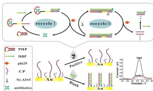
**Fig. 1** Schematic illustration of antibiotics assay using target-aptamer binding triggered quadratic recycling amplification strategy.
