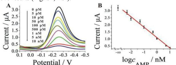
**Fig. 4** (A) Typical DPV responses of the biosensor to different concentrations of AMP; (B) The calibration curve of DPV peak current versus the logarithm of AMP with various concentrations. Error bars are standard deviations across four repetitive experiments.
