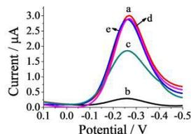
**Fig. 2** Typical DPV responses of target-triggered quadratic recycling amplification via the exposure of the modified electrode to blank sample (a), positive sample (10 nM AMP, b), 10 nM AMP without *Nt.AlwI* (c), 10 nM AMP without phi29 (d), 1 μM penicillin in place of AMP (e).
