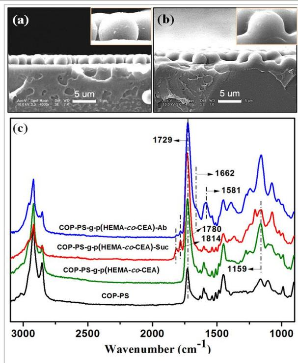
**Fig. 1** SEM images of the cross sectional view for COP-PS supports (a) before and (b) after photografting polymerization, (c) ATR-FTIR spectra of the samples.
