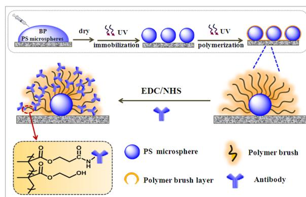
**Scheme 1.** Preparation of microsphere-polymer brush hierarchically 3D substrates via a two-step UV irradiation procedure.
