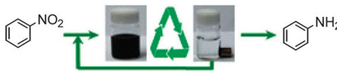
Fig. 23 Heterogeneous reduction of nitrobenzene with hydrazine using magnetically recyclable hollow nanocomposite catalysts. Catalyst separated by a magnet kept in contact with the bottle from outside.
