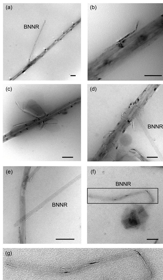
**Fig. 2** TEM images of peeled BNNTs produced in (a) PrOH, (b) BuOH, (c) PeOH, (d) HeOH, (e) BNNRs with pristine straight edges produced in BuOH, (f) twisted BNNRs produced in BuOH, and (g) the magnified image of the framed region in (f). All scale bars represent 100 nm.
